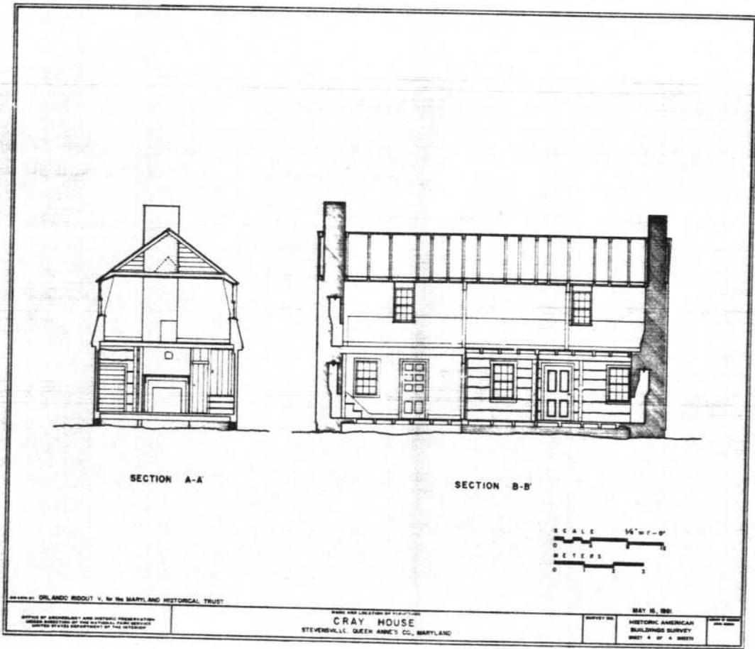
steeply pitched gable roof was replaced with the present gambrel roof. The outline of an early frame kitchen, now demolished, can be seen in the north gable of the main house.
